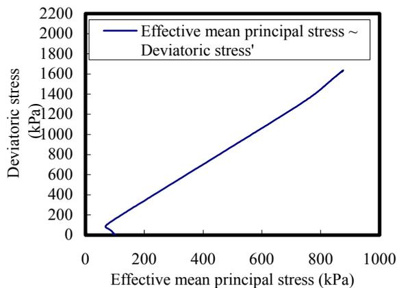
Figure 2.3.3  $p' \sim q$  curve [Effective stress path]
