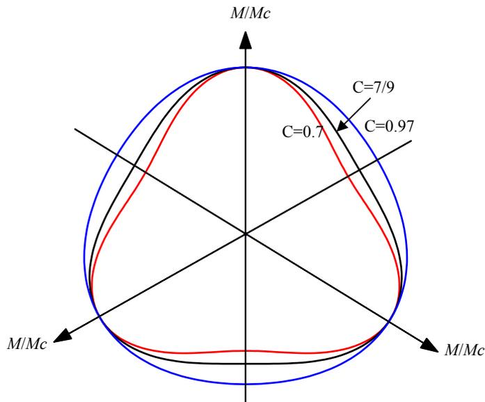
Figure 2.2.1 Yield surface shapes on  $\Pi$  plane depending on the parameter  $C$
