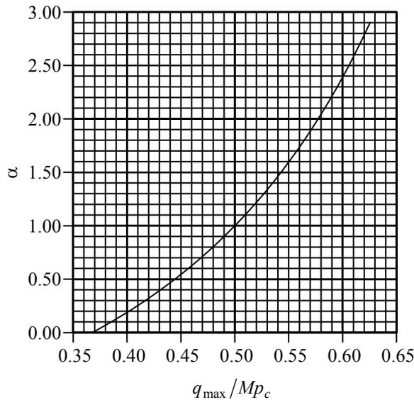
Figure 3.2.2  $\alpha$  and  $q_{\max}/Mp_c$  of normally consolidated clays from  $\overline{CU}$  test
