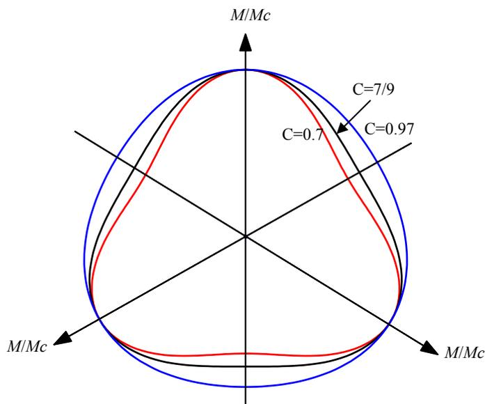
Figure 3.2.1 Yield surface shapes on  $\Pi$  plane depending on the parameter  $C$
