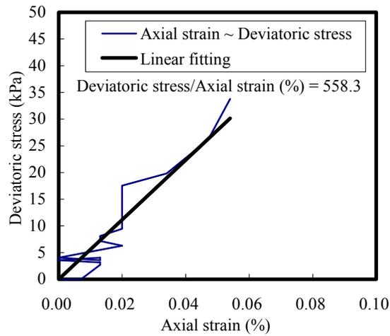
Figure 2.3.5 Young's modulus  $E_t = 55,830\text{kPa}$  from the initial slope of  $\varepsilon_a \sim q$  curve
