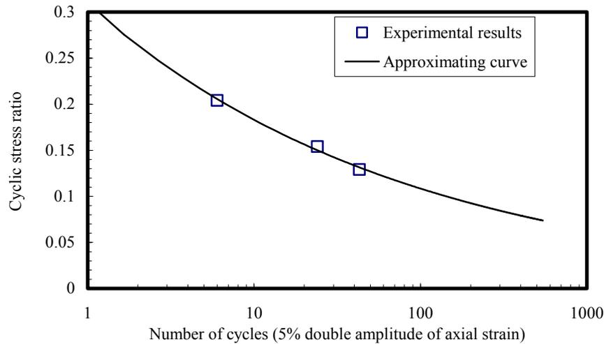
Figure 2.3.14 Liquefaction strength of experimental results from cyclic undrained triaxial test
