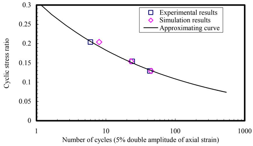
Figure 2.3.15 Liquefaction strength of simulation results from cyclic undrained triaxial test
