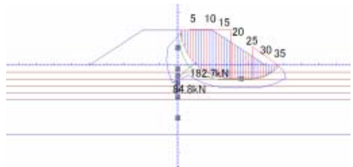
Figure 8. A non-arc by limit equilibrium method slips.
