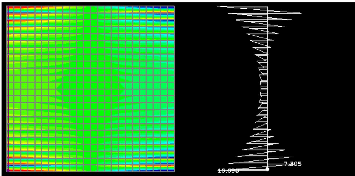
Figure 5: Intra element out of plane shear oscillations (raw)
