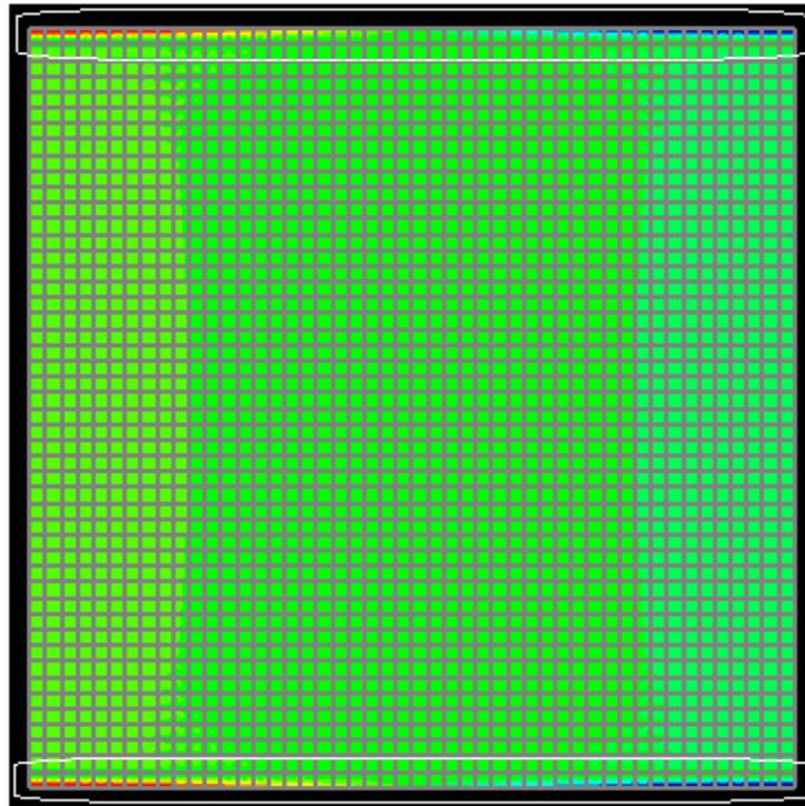
Figure 3: Stress concentrations in a simply supported plate (smoothing enabled)
