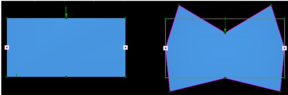
Figure 1: Zero energy mode in static analysis
